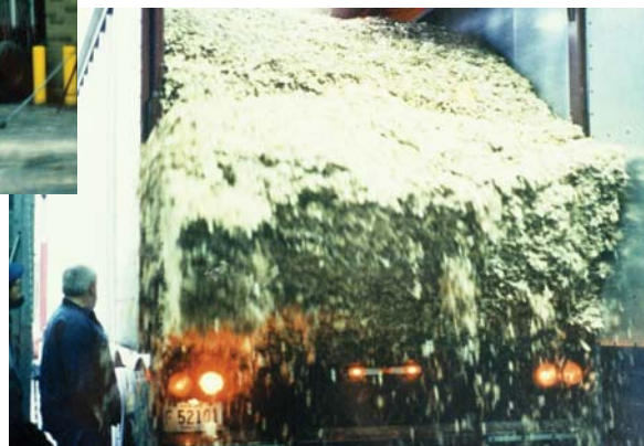
Mountain View School, Kingsley, Pennsylvania Facility Type: Two schools on adjacent properties System Size: 9.5 MMBH Manufacturer: Sylva Energy Systems Showing chip delivery from self-unloading tractor-trailer van.
